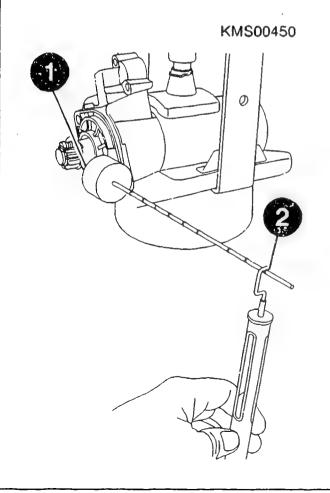
Checking armature braking torque
